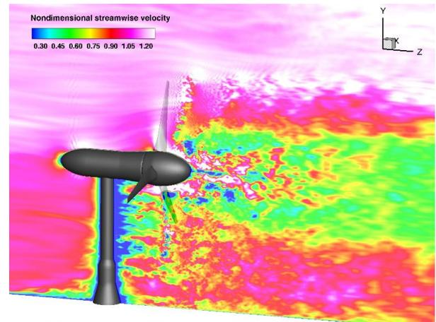
Figure 2: LES of flow past a hydrokinetic turbine on a grid with 150 million nodes.  $Re=237,000$ , tip speed ratio=4.7,  $F_r=0.14$ . The turbine is mounted on the bottom of a rectangular open channel. Hub height is  $0.8D$  and channel depth is  $2.3D$ . F. Sotiropoulos, Univ. of Minnesota.
