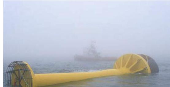
Figure 10: Float-out foundation (MBD Ocean Power)
