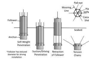
Figure 3. The installation procedure of the MRA
