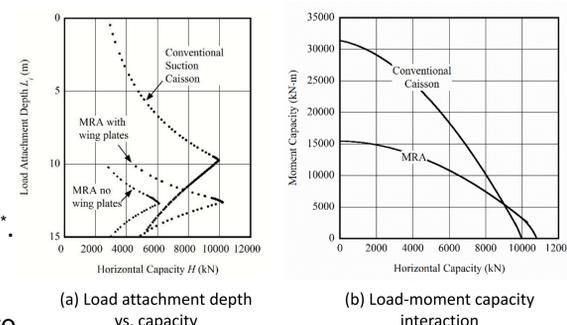
Figure 5. Horizontal load capacity of MRA in clay
