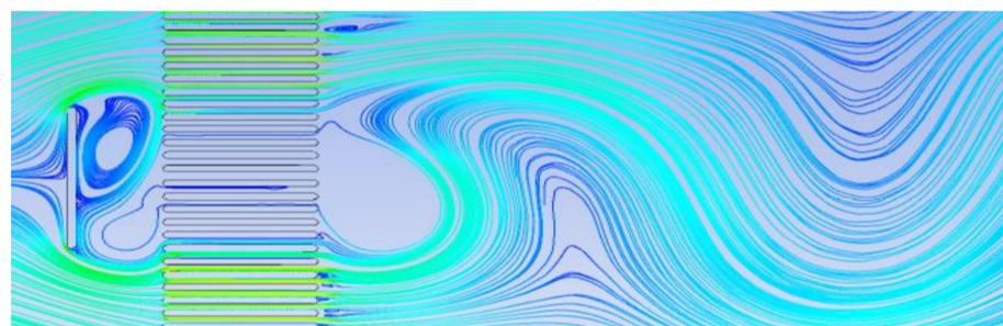
Fig.5 Vortex Street Formed behind Honeycomb
