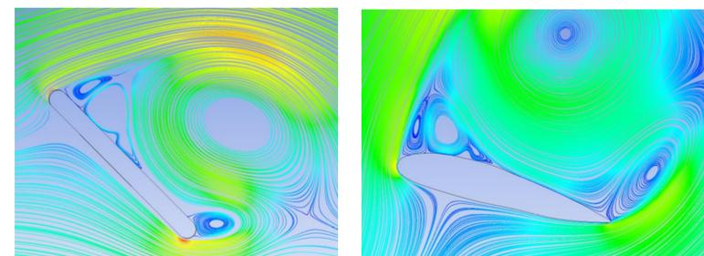
Fig.2a Inclined Plate @  $\alpha = 45^\circ$
