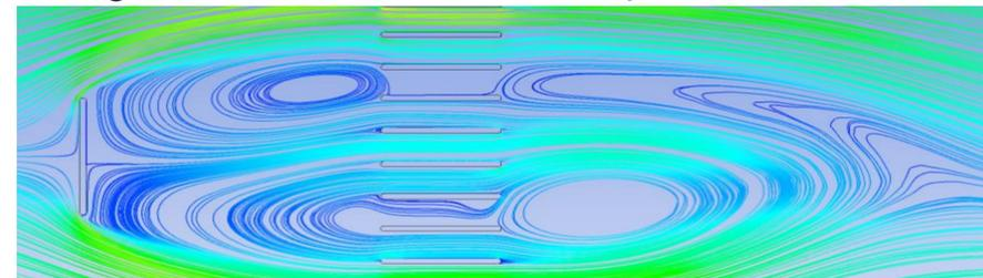
Fig.3a Shed Vortices Approaching Coarse Honeycomb
