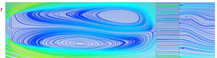
Fig.4 Shed Vortices Stretched Between Flat Plate and Honeycomb
