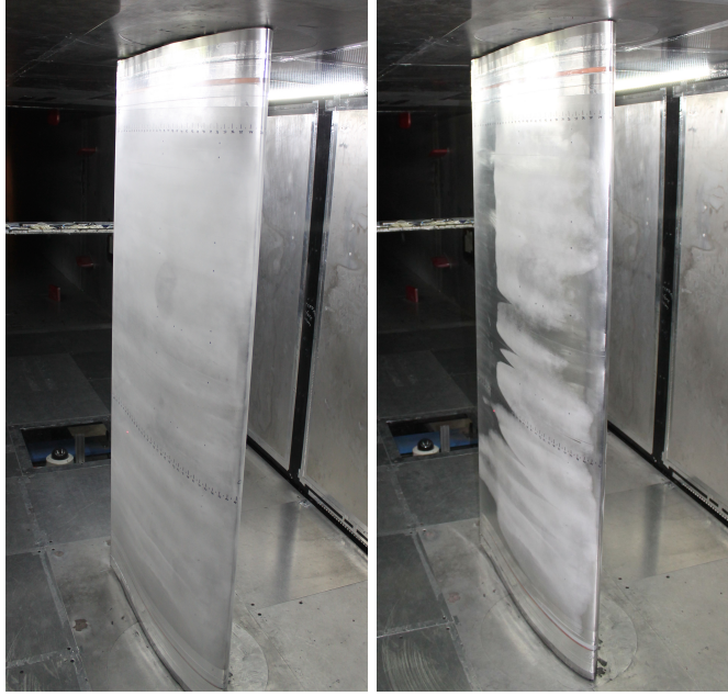
Figure 1: Naphthalene visualization on pressure side of the DU96-W-180 model at \alpha = 8^\circ and Re_c = 3.0 Million. Left: after naphthalene application. Right: after wind tunnel was held on condition for \sim 10 minutes and turned off.
