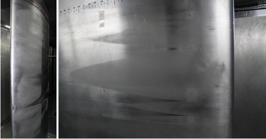
Figure 2: Naphthalene visualization on the DU96-W-180 model at Re_c = 3.0 Million. Left: suction side at \alpha = 0 degrees, flow from left to right. Right: pressure side at \alpha = 8 degrees, flow from right to left. Turbulent wedges caused by forty-micron-thick tape and surface defects at laminate edges.
