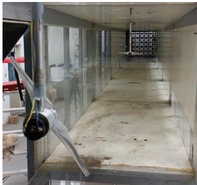
Figure 4. Wind Turbines in array with 10 diameters of distance between them.
