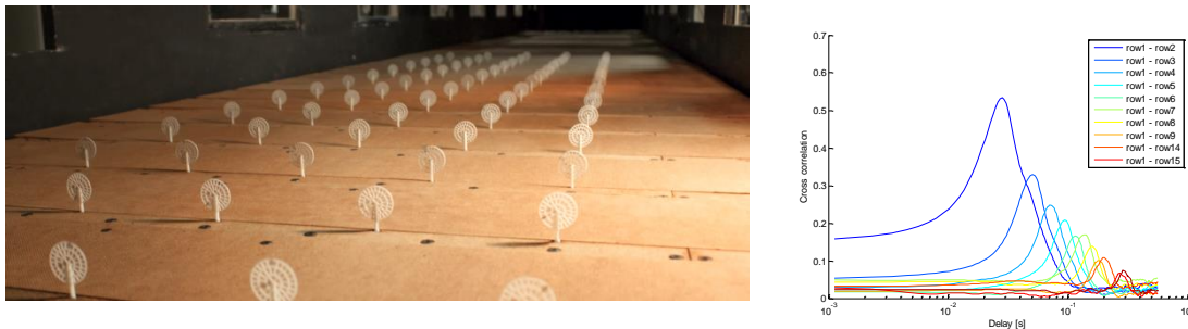
Fig. 2 Micro wind farm set-up (Left). Cross correlation between the thrust force of stream wise aligned wind turbine models (right).
