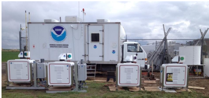
Fig. 1 Scanning Doppler wind LiDARs deployed for the XPIA experiment.
