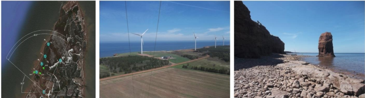
Fig. 1 Left: Overview of the site showing the 5 DeWind 2 MW turbines (cyan), ZephIR lidars (green), IEC compliant MM (green open circle) and the Galion (red dot). Center: Photograph from the 80-m MM looking northwest. T4 is shown in the center of the image. Z447, a Gill sonic and an 18-m MM were located west of T4 (towards the cliff). Photo: André Doucette. Right: Photograph of the escarpment looking south. Photo: Sara C Pryor.
