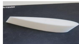
Fig. 2 Airfoil's blade produced on 3D printed with precision of 0.3mm (layer height)
