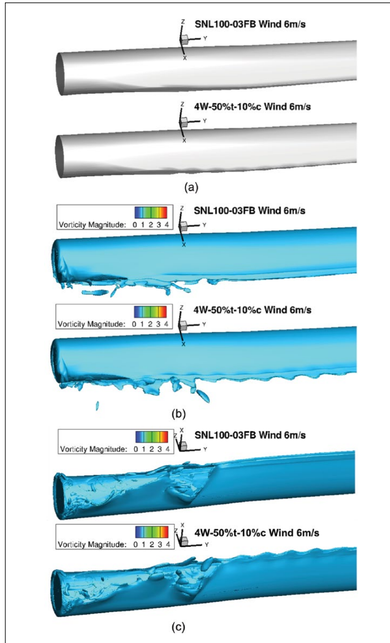
Figure 21. Iso-vorticity magnitude at the blade inboard: wind speed of 6 m/s: (a) geometry, (b) upper surface view, and (c) lower surface view.
