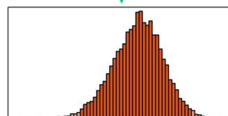
Distribution of flutter speed is predicted by including various **uncertainty** sources (aerodynamic loads, structural properties, etc.)
