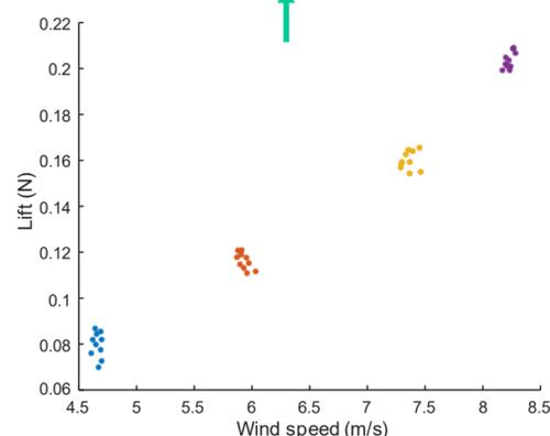
Aerodynamic loads are determined through wind tunnel tests accounting for **experimental variability** (example: lift measured in NEU's wind tunnel)
