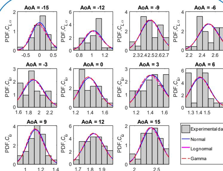
(Example) Empirical histogram of  $C_0$ , compared with fitting distribution models
