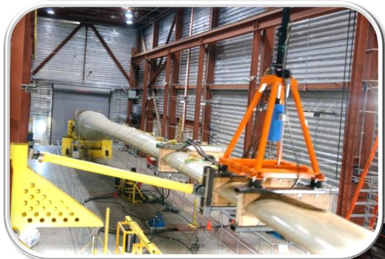
NREL (CO) – drive train & blade test
