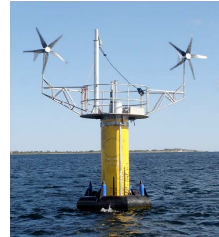
Floating wind LIDAR; The Natural Power Sea Zephyr (from http://blog.lidarnews.com )
