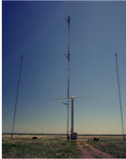
Figure 2 - NREL Long-Term Inflow and Structural Testing (LIST) Program (see Kelley et al. (2002) for details). Inflow turbulence measurement array looking downwind towards the NWTC 600-kW CART turbine. Photo by Warren Gretz (NREL).
